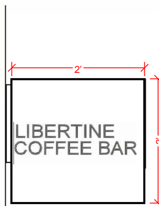
2 WALL SIGN (LOGO SOUTH) 3/4" = 1'-0" * SIGN TO BE METAL EXTERIOR ILLUMINATED. ATTACH PER MANUFACTURER SPECIFICATIONS.
