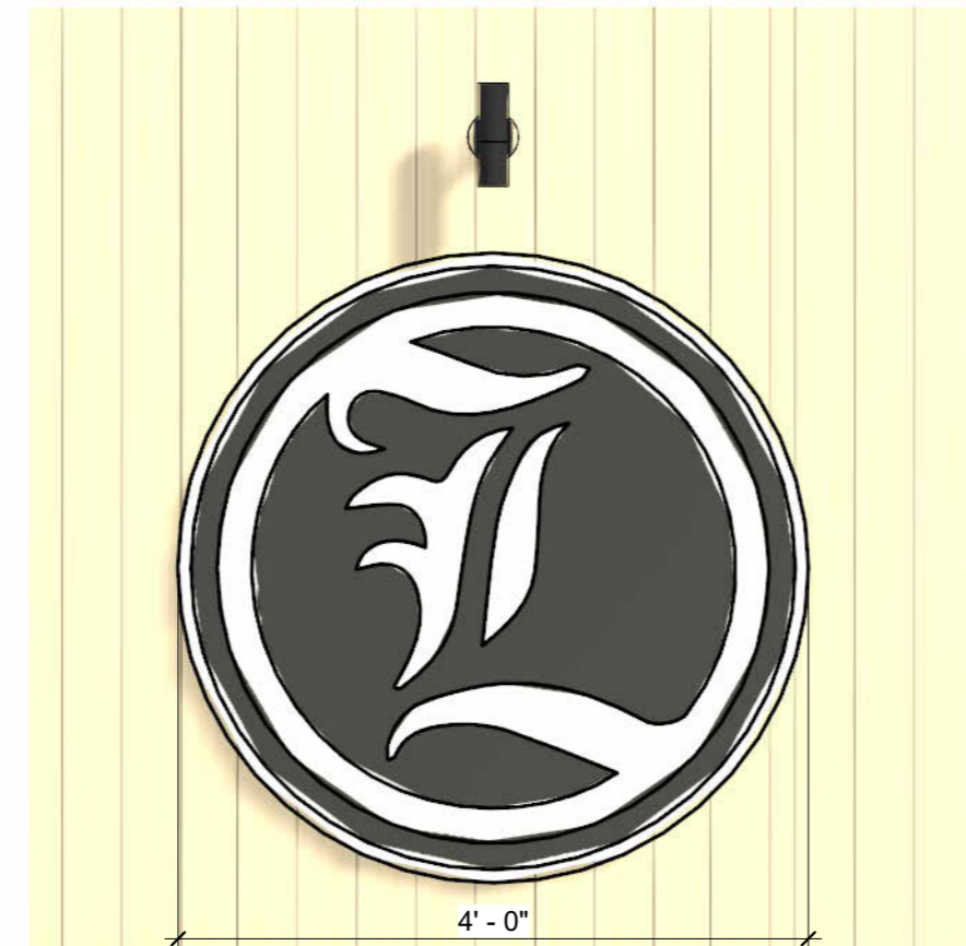
2 WALL SIGN (LOGO SOUTH) 3/4" = 1'-0" * SIGN TO BE METAL EXTERIOR ILLUMINATED. ATTACH PER MANUFACTURER SPECIFICATIONS.
