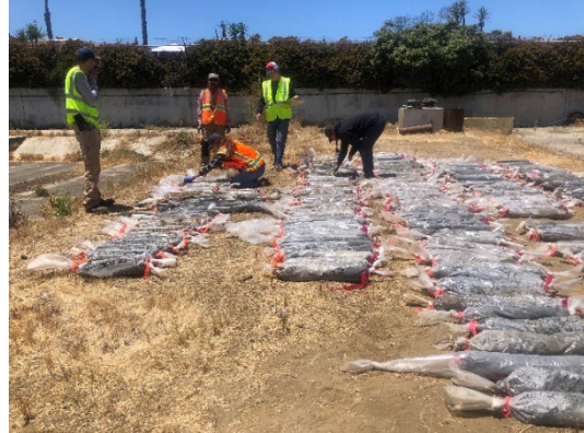
Well Site Cores (Deep Sonic Cores)
