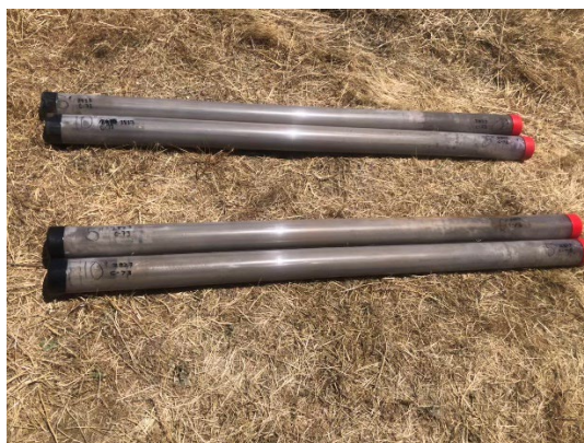
Pipeline Alignment Cores (Shallow Cores)
