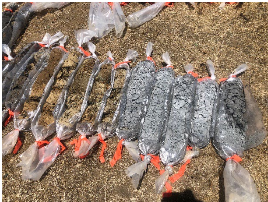
Well Site Cores (Deep Sonic Cores)
