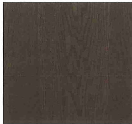
WOOD HEADERS, RAFTER TAILS & DECK CEILING FINISH (DARK WALNUT STAIN)
